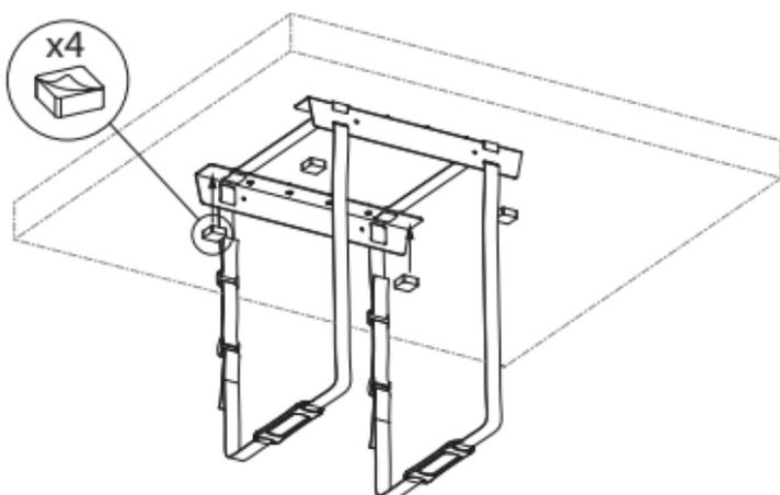
Attach the Stopper 02 to the Holder 01 as the above diagram.
