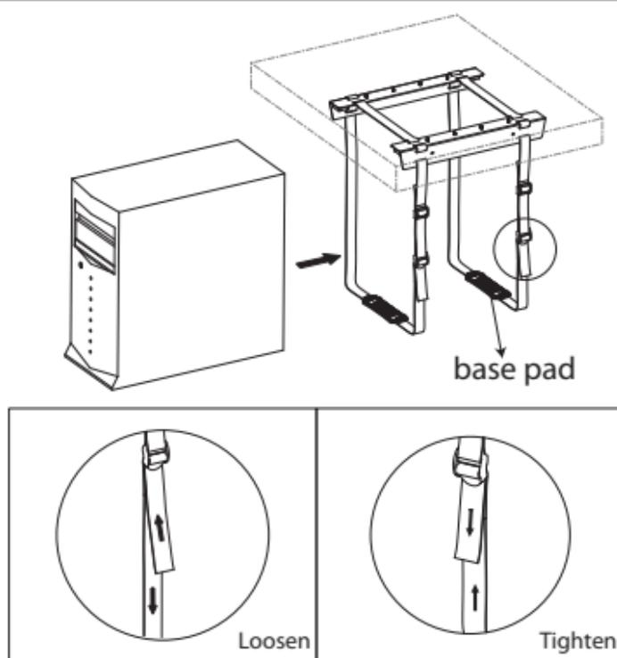
Attach the PC tower to the Holder 01 and make sure the base pads placed in the middle of PC tower bottom. Adjust the webbing to fasten the PC tower stably on the Holder 01.
