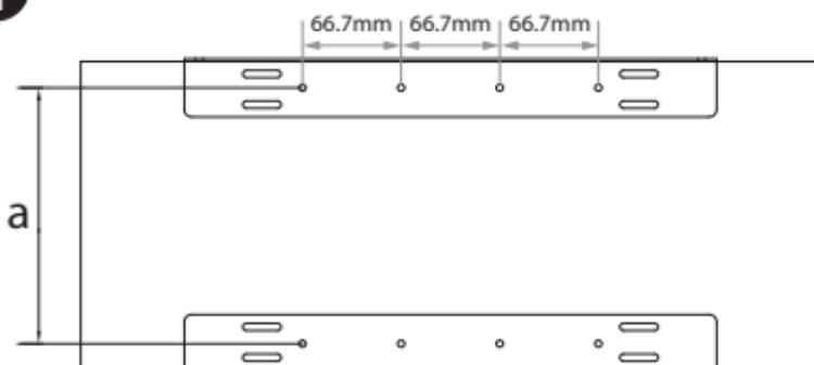
Place Holder 01 on top of PC tower as the above diagram. Measure the distance "a" by the tape. Make 8 marks under the desk as the below diagram for the location you want to install this PC tower holder.
